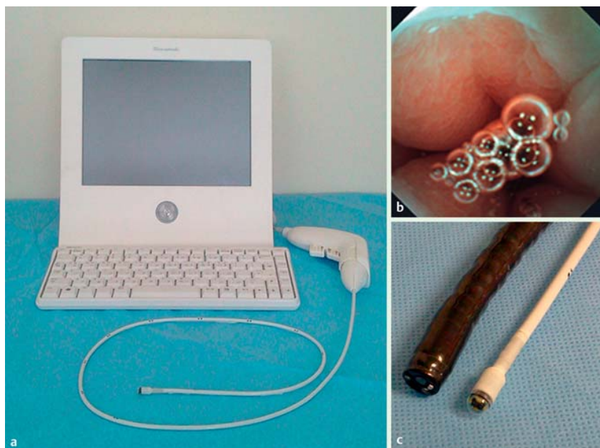
Fig. 1 E.G. Scan system. a E.G. Scan display system, controller, and probe. b E.G. View. c Relative diameters of two endoscopes, the E.G. Scan (6 mm) and a conventional endoscope (9.8 mm, GIF-H260, Olympus Optical, Ltd., Tokyo, Japan).
